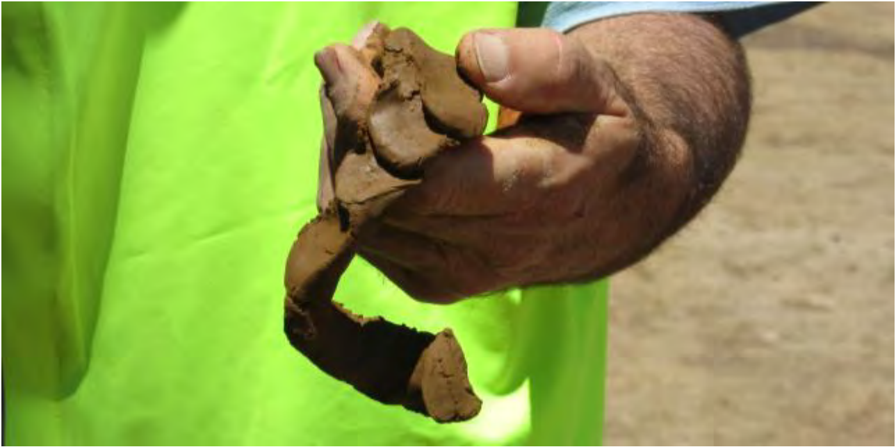
Photo 4: A long ribbon can be moulded from a sample of the IIB horizon (from the site 1 subsoil), demonstrating its high clay content.
