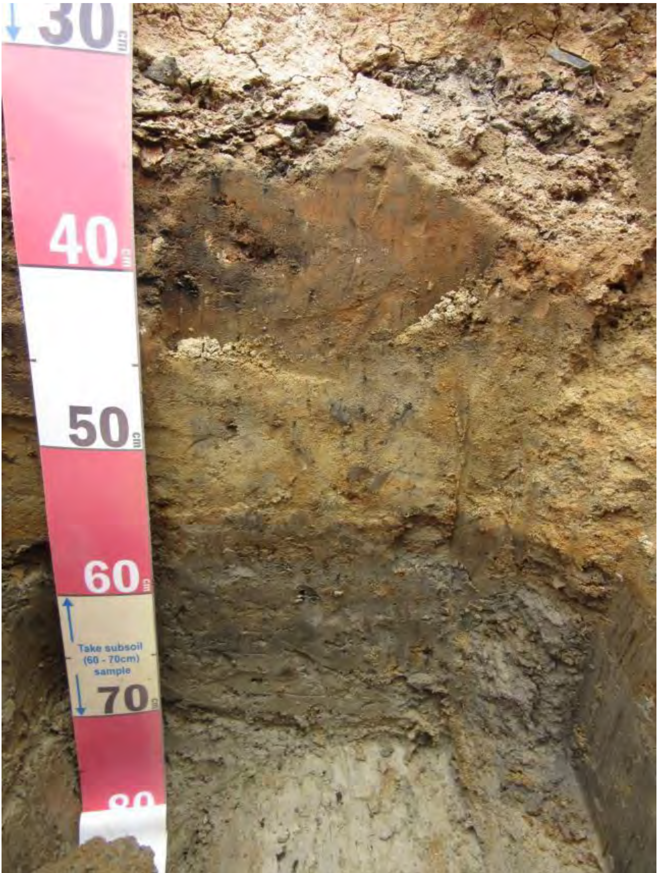
Photo 7: The Casey & Lowe test trench 18 soil profile has dark clayey fill covering another fill layer of yellowish light brown sand (between 45 and 55 cm depth) that has protected the grey historic topsoil underneath it. On the floor of the pit is a pale grey silty light clay, the A 2 horizon of the original profile. Its chemical properties have remained unaffected by British settlement.
