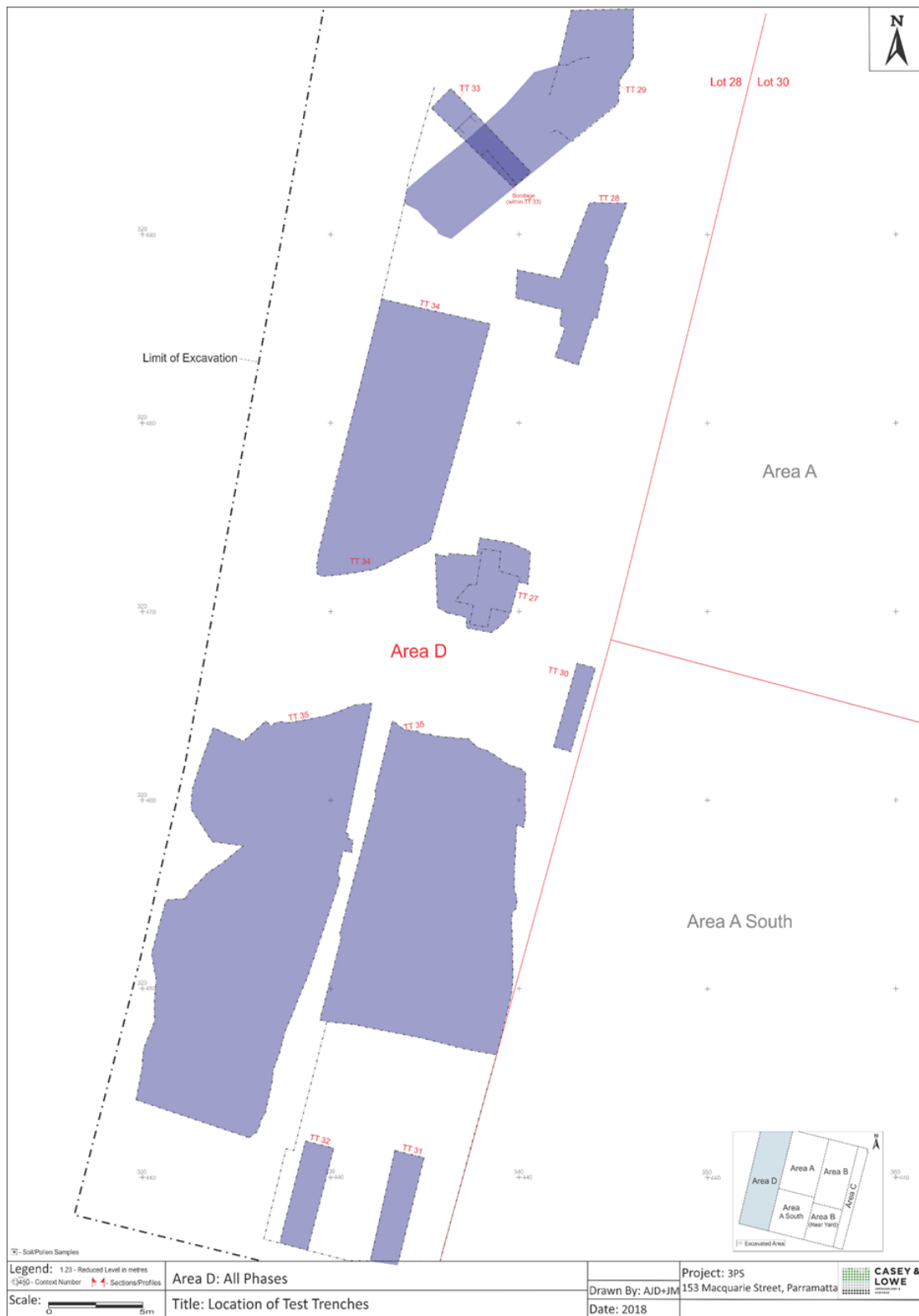
Figure 3.1: Plan showing the location of the various test trenches excavated by machine and then manually across Area D (shaded). The trenches to the north were generally deeper than those to the south, except for the machine excavated trenches through the pond TT31 and TT32. The western edge of the site to the north was under the footpath full of services so it was not investigated.
