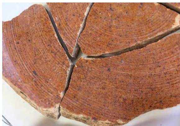
Figure 5.11: Detail of manufacturing fault of iron spots in the glaze, on milk pan 17568/#47676. B McCall.
