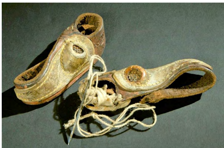
Figure 4.96: Sailor's palm gloves with circular thimbles. Made by Shrimpton & Sons, Reddich, UK. 113
