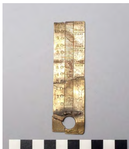
Figure 4.50: Brass thermometer backplate with graduated Fahrenheit scale and comparative heat indications 17545/#539. 100mm scale. Gallery2. IMG_4208.
