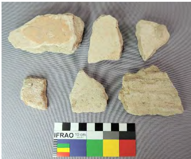
Figure 4.5: Sample of 2-coat plaster render painted salmon pink on/ white (3+ coats). Bottom right: back showing lath impressions. 100mm scale. Casey & Lowe. DSCN8065.
