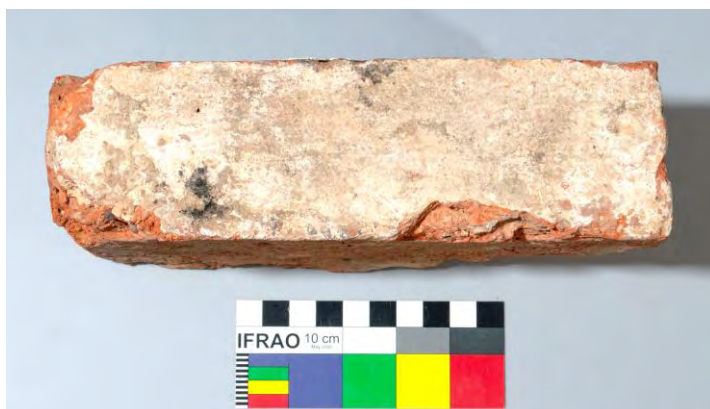
Figure 4.63: Flat (slop) sandstock brick with whitewashed side, other with soot, from Room 4 fireplace demolition rubble 16159/#8628. 100mm scale. Gallery2. IMG_4245.
