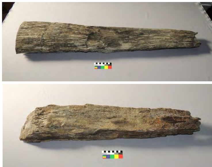
Figure 3.52: Two timbers from the timber barrier 17853 showing the chamfered wedge-shaped base. Narrow-leaved Red Iron Bark ( Eucalyptus ? crebra ). DSCN3713, DSCNS3727, scale 100mm.
