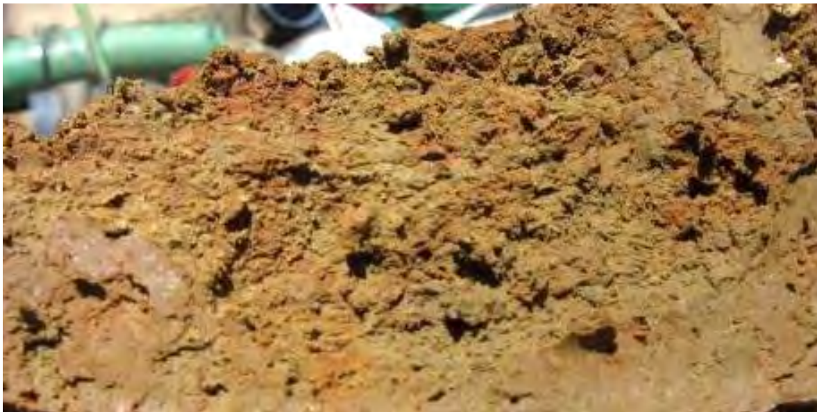
Figure 3.20: Dense yellowish brown clay subsoil (from the IIB horizon) with reddish brown mottles, from a depth of 20-25 cm at site 1. Clay similar to this was seen at several locations, usually at shallow depths, across the whole site. Roy Lawrie Soil Report, 2019, Vol. 3. Sec. 8.6.
